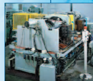
Tester for bearings used in work rolls of rolling mills
