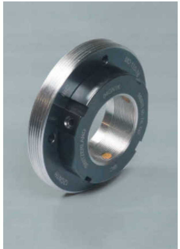
Fig. 7.12: Compact combination of precision seal ring locknut MD with outer thread to set the bearing outer rings and precision labyrinth groove nut MMRS to preload the inner rings and simultaneously the self-locking seal
