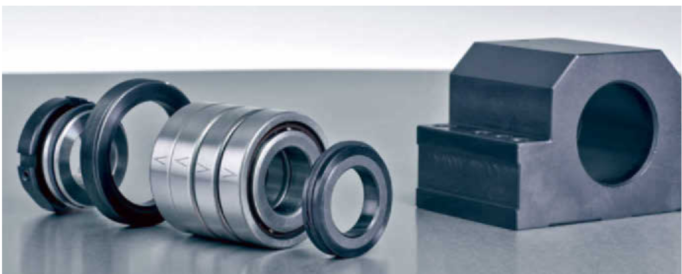
Fig. 2.1: Components of an IBC precision pillow block unit BSPB-M, consisting of a precision locknut MMRS and a precision seal ring locknut MD, four single-row 60° ball screw support bearings, precision labyrinth seal S and precision pillow block housing
