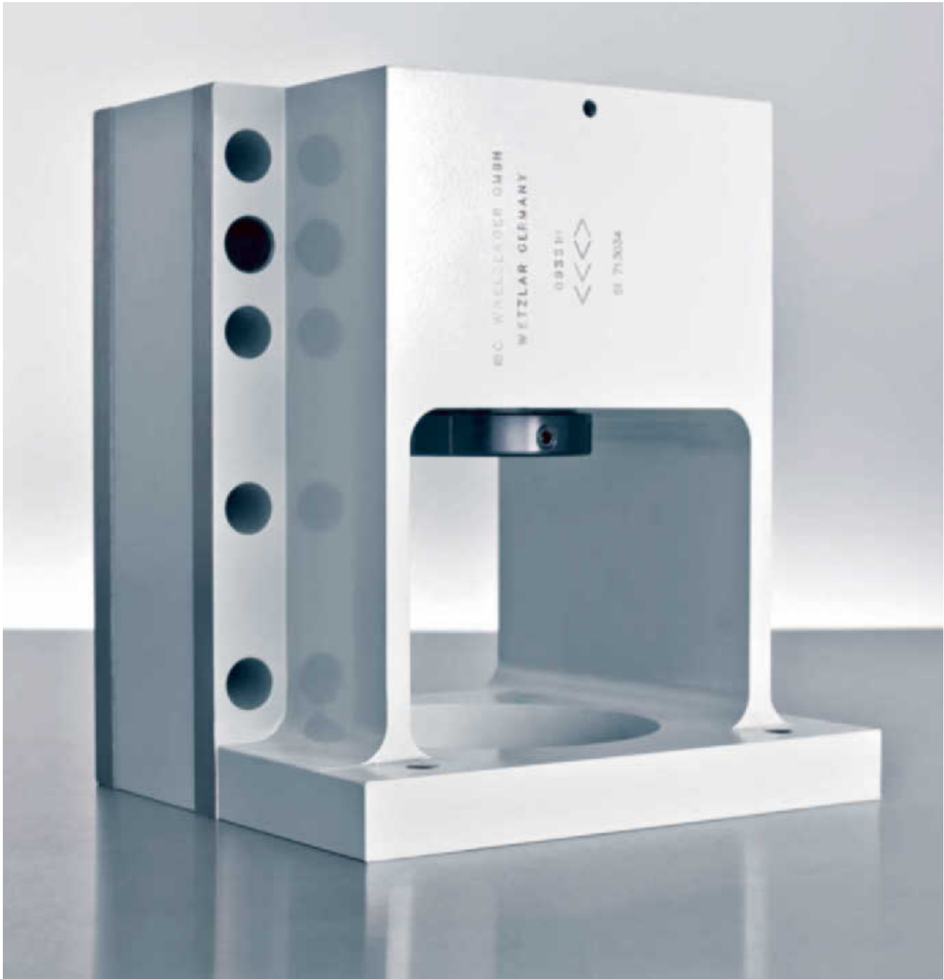
Fig. 5.21: Easy to install IBC precision special pillow block unit with asymmetrical bearing arrangement for vertical axes, motor flange integrated underneath - painting of the housing optional
