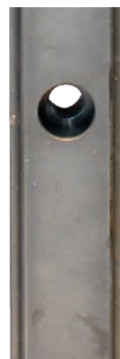
Rail with CTS coating – after 22 hours of salt spray test (acc. to DIN EN ISO 9227)
